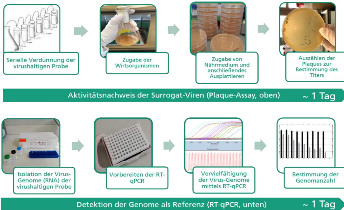
Figure 14: Culture-based detection of viral infectivity (top) and molecular analysis of the number of viral genomes (bottom), which can be used to evaluate the effectiveness of indoor air purifiers
