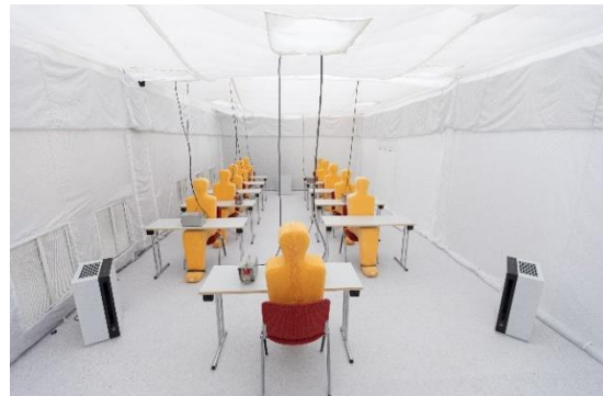
Figure 2: Setup for evaluating mobile air purifiers with the aid of virus surrogate aerosols (left) and surrogate DEHS aerosols (right) at Fraunhofer IZS in Stuttgart
