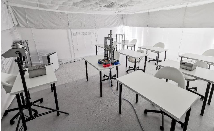
Figure 13: Test set-up for evaluating mobile air purifiers with virus surrogate aerosols at STEP Stuttgart Engineering Park in Stuttgart Vaihingen.
