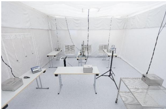
Figure 2: Setup for evaluating mobile air purifiers with the aid of virus surrogate aerosols (left) and surrogate DEHS aerosols (right) at Fraunhofer IZS in Stuttgart
